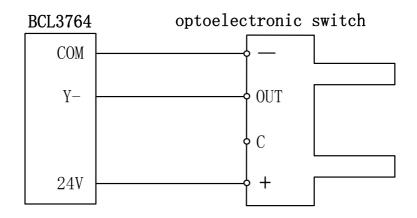
Typical connection of contact switch is shown as below:
