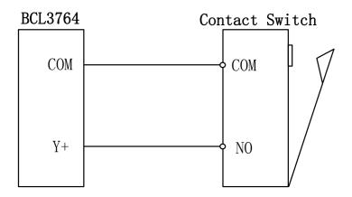
Typical connection of magnetic switch is shown as below, which must use 24V switch of the NPN type.
