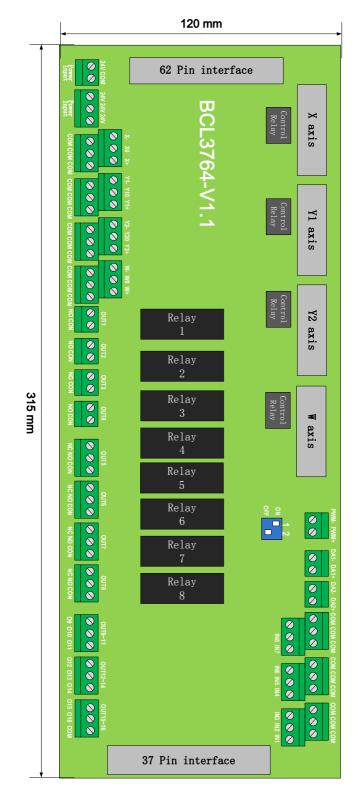
BCL3764-V1.1 external IO board is installed by rail and also can be installed permanently. Its external size is 315mm\*107mm with DM62M and DB37M interface
