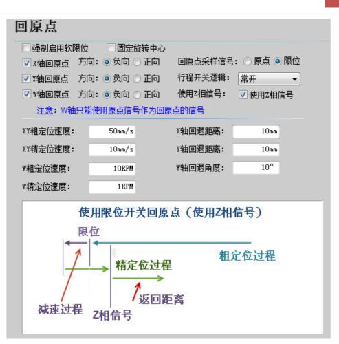
As long as conditions allow, be sure to select "Use Z-phase signal", which will greatly enhance the accuracy of homing origin. BMC1205 motion control card matched with CypTube provides encoder input to each axis, to extremely ensure accuracy.
