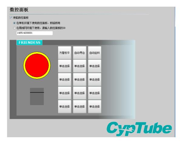
BCP5045 numerical control panel can be activated in numerical control panel interface. When used in a stand-alone environment, CypTube software will adaptively match the Mac address of BCP5045 numerical control panel, and automatically connect the control. When BCP5045 is used in the LAN environment, please enter BCP5045 device ID number. BCP5045 is in total of 12 custom keys, which can be configured as a control button of double exchange workbench or other custom PLC.
