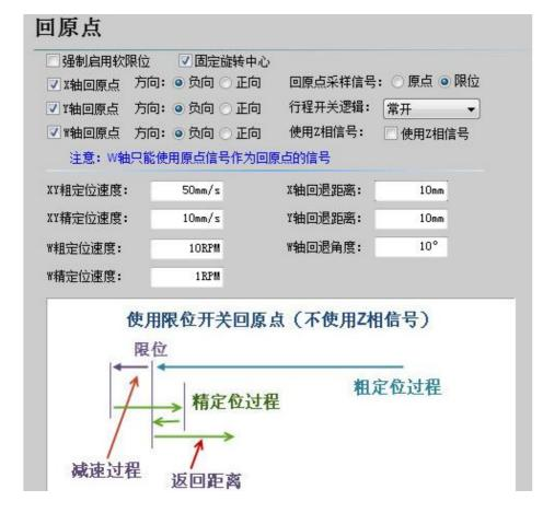
**Forced open software limit:** Enforce to Open soft limit function, and prevent users from manually switching the soft limit in the master interface of CypTube.
