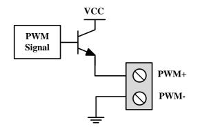
We strongly recommend that users install PWM+/- signal to a relay output port in series (PWM+/- enabled), then access to the laser, which can avoid laser light leakage in modulation mode. Please refer to "2.5 Laser Connection" for more details. Furthermore, please adjust PWM signal level. 24 V or 5 V level can be selected through dip switch.
