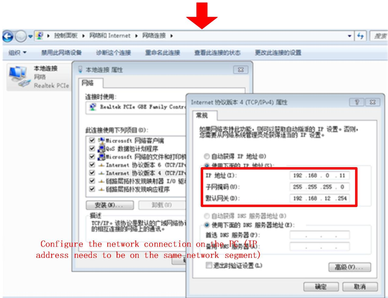
Figure 10 Ethernet connection steps
