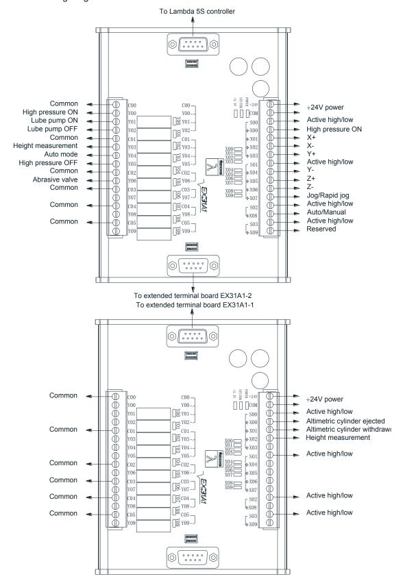
Fig. 2-30 Wiring example of extended terminal board EX31A 1in case of five -axis waterjet cutting machine of AC-type
