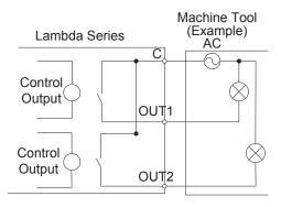
Fig. 2-59 Connection of relay output with contactor
