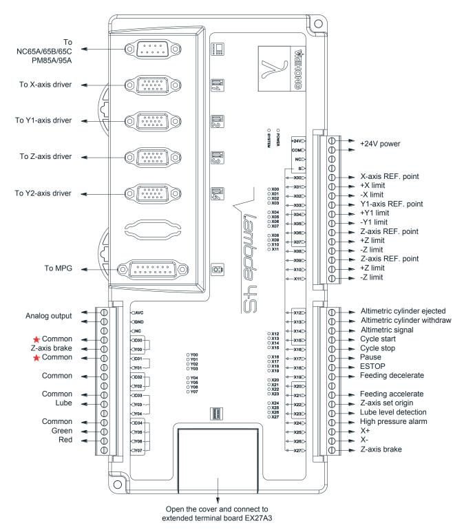
Fig. 2-17 Wiring according to XY1ZY2 configuration according to waterjet cutting software
