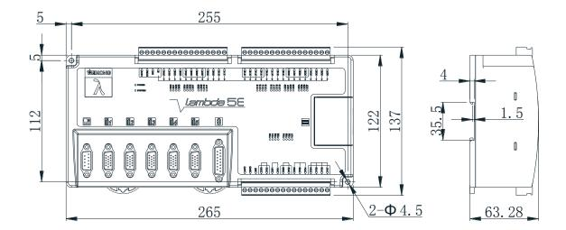
Fig. 1-7 Dimensional drawing of Lambda 5E controller
