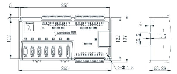
Fig. 1-6 Dimensional drawing of Lambda 5S controller
