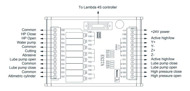
Fig. 2-18 Wiring of EX27A according to XY1ZY2 configuration according to waterjet cutting software
