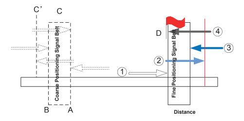
Fig. 6-3 The process of fine positioning
