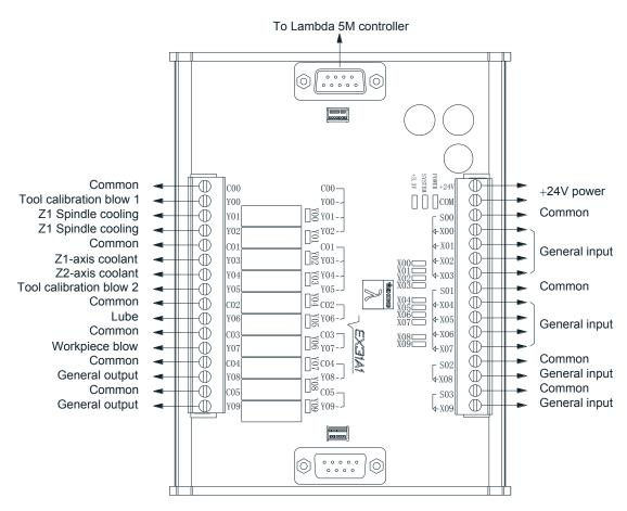
Fig. 2-48 Wiring of EX31A1 in dual Y union configuration of NK300CX software (multi Z)
