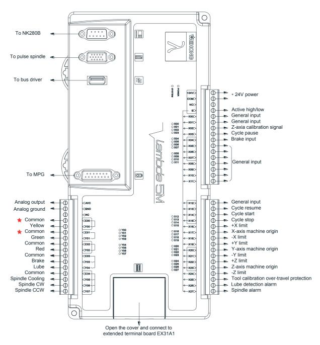
Fig. 2-39 Wiring of Lambda 5M in NK280B integrated CNC system
