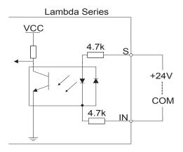
Fig. 2-58 Binary input connecting with mechanical switch
