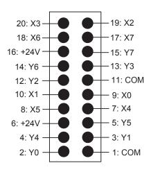
Fig. 2-57 Non-cascade connection type extended terminal board interface
