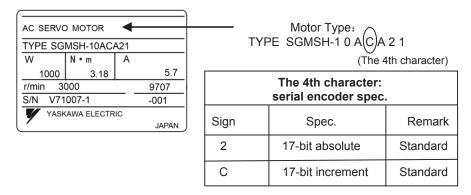
Fig. 6-9 Name plate of servo motor-encoder resolution
