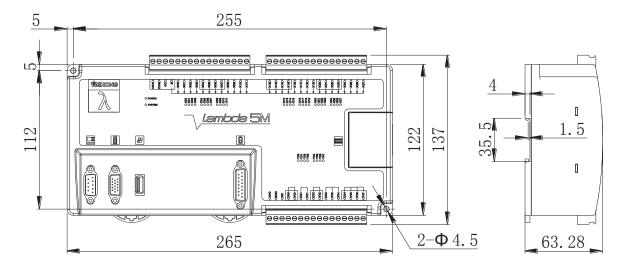
Fig. 1-8 Dimensional drawing of Lambda 5M controller
