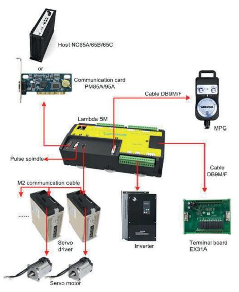
Fig. 1-10 Overall wiring diagram (bus system)
