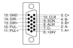
Fig. 2-54 Definition of driver interface
