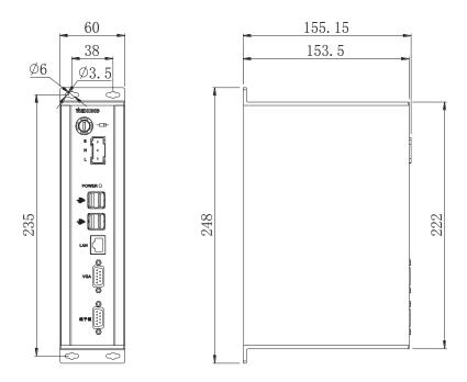
Fig. 1-2 Dimensional drawing of NC65B host
