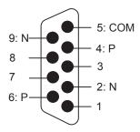
Fig. 2-56 Cascade connection type extended terminal board interface
