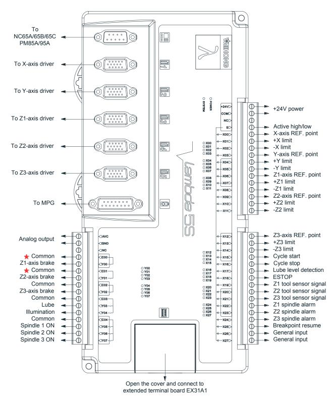
Fig. 2-35 Wiring according to three Z axes software
