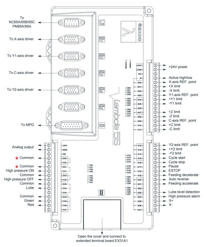
Fig. 2-21 Wiring according to XY1CY2 configuration according to waterjet cutting software
