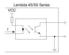
Fig. 2-60 Output circuit of servo enable signal
