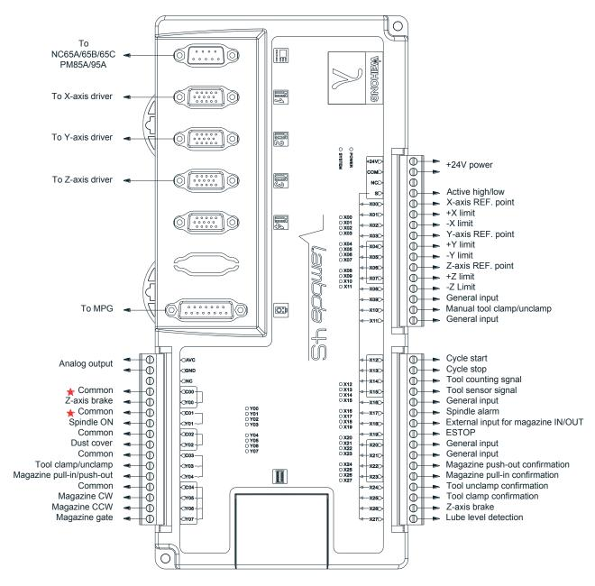
Fig. 2-3 Wiring according to three-axis disk-type tool magazine configuration according to engraving and milling software
