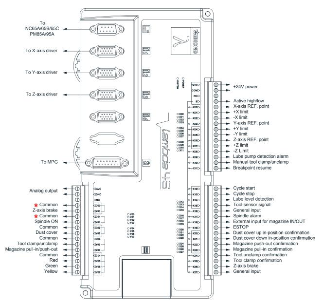
Fig. 2-4 Wiring according to three-axis linear tool magazine configuration according to engraving and milling software
