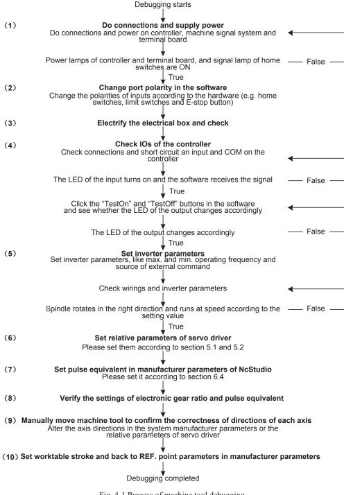
Fig. 4-1 Process of machine tool debugging
