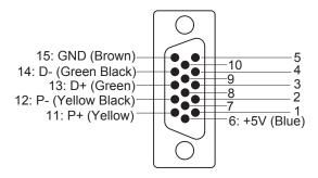
Fig. 2-53 Definition of driver interface
