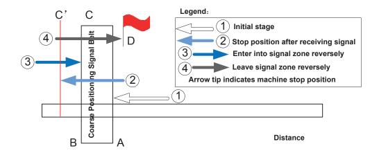
Fig. 6-2 Sketch map of coarse positioning (stopping out of the signal belt after receiving REF. point signal)
