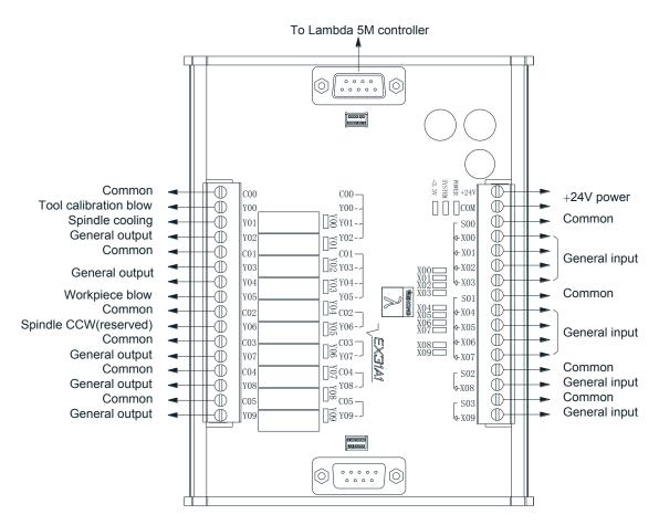
Fig. 2-42 Wiring of EX31A1 in NK300CX software (integrated)
