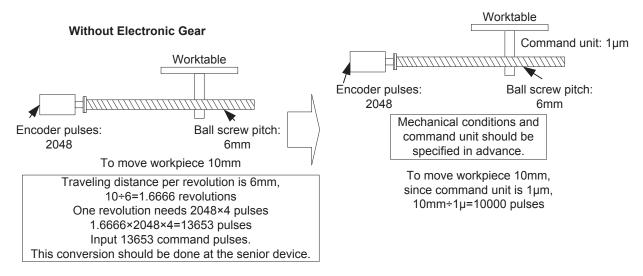
Fig. 6-10 Schematic conversion of electric gear ratio
