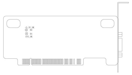
Fig. 1-3 Structural drawing of communication card PM85A
