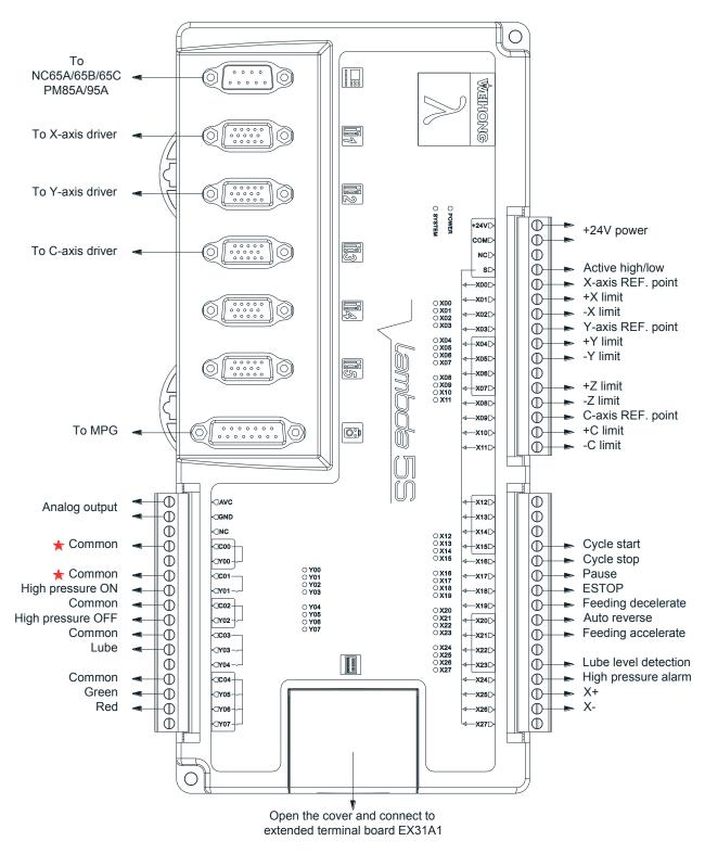
Fig. 2-19 Wiring according to XYC configuration according to waterjet cutting software
