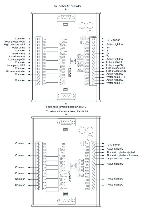
Fig. 2-26 Wiring example of EX31A1according to XY1ZCY2 configuration according to waterjet cutting software
