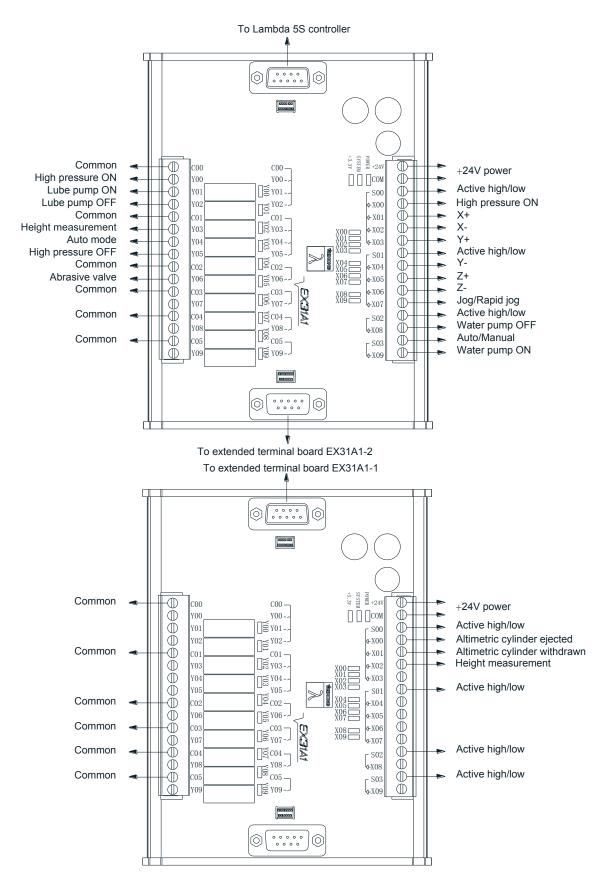
Fig. 2-28 Wiring of EX31A1 according to StadA with 2Y configuration according to waterjet cutting software
