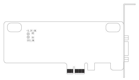
Fig. 1-4 Structural drawing of communication card PM95A
