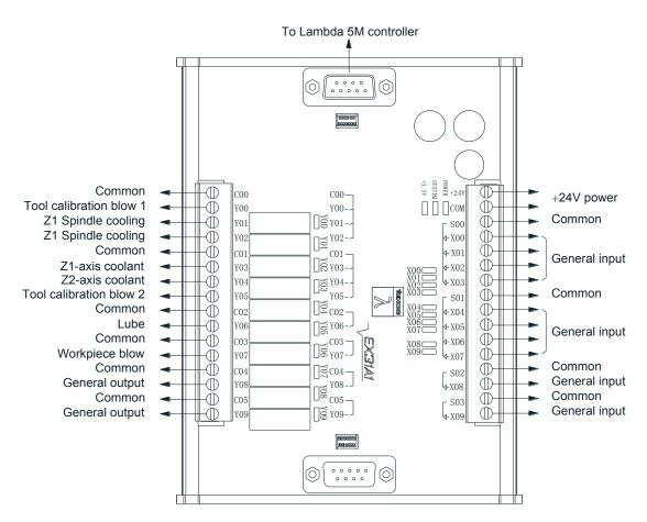
Fig. 2-44 Wiring of EX31A1 in union configuration of NK300CX software (multi Z)
