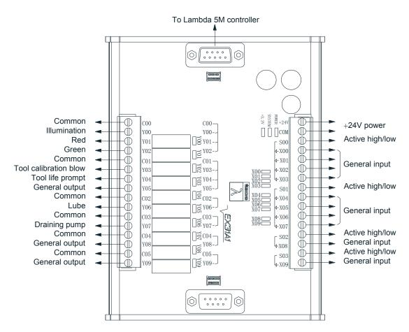
Fig. 2-50 Wiring of EX31A1 according to three-axis dual Z NcStudio V10 software
