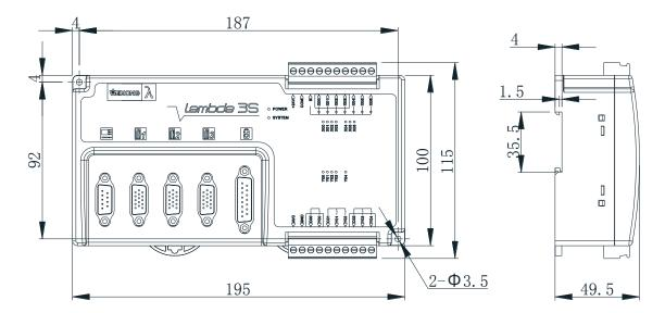
Fig. 1-5 Dimensional drawing of Lambda 3S
