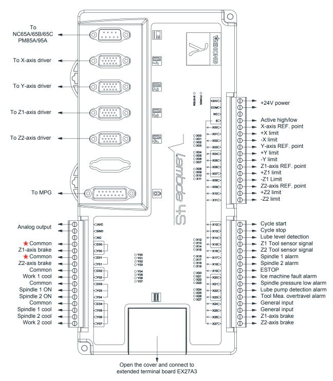
Fig. 2-33 Wiring according to dual Z axes software
