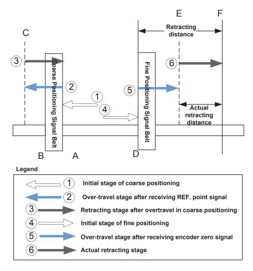
Fig. 6-5 The process of returning to machine origin
