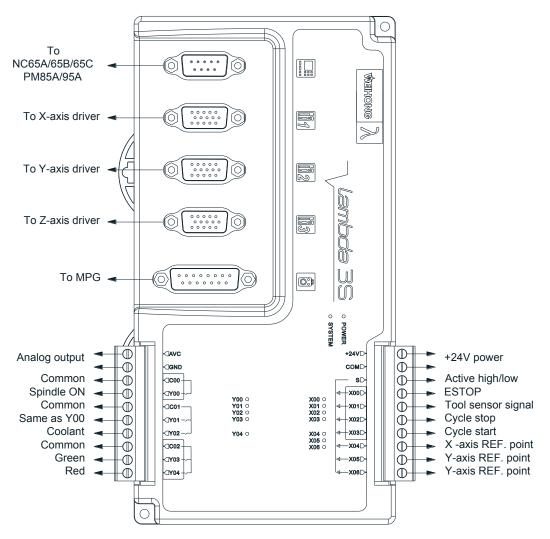
Fig. 2-1 Wiring of Lambda 3S controller
