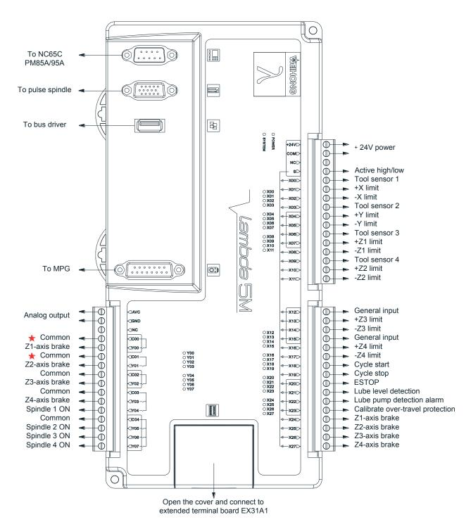
Fig. 2-51 Wiring of Lambda 5M in three-axis Quadruple Z NcStudio V10 software
