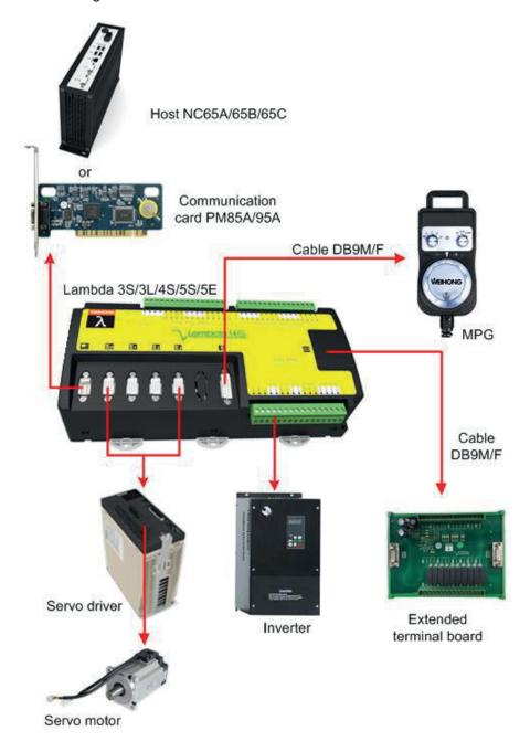
Fig. 1-9 Overall wiring diagram (non-bus system)
