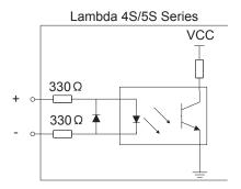
Fig. 2-61 Input circuit of encoder signal
