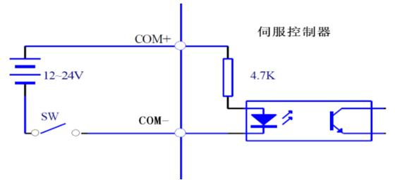
Figure 4.3-a Input Interface for Switching Value
