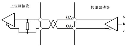
Figure 4.6 CN1 Output Interface for Encoder
