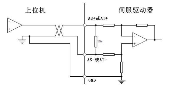
Figure 4.5-a Interface for Analog Differential Input
