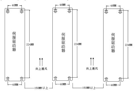
Figure 1.3 Direction of Installation
