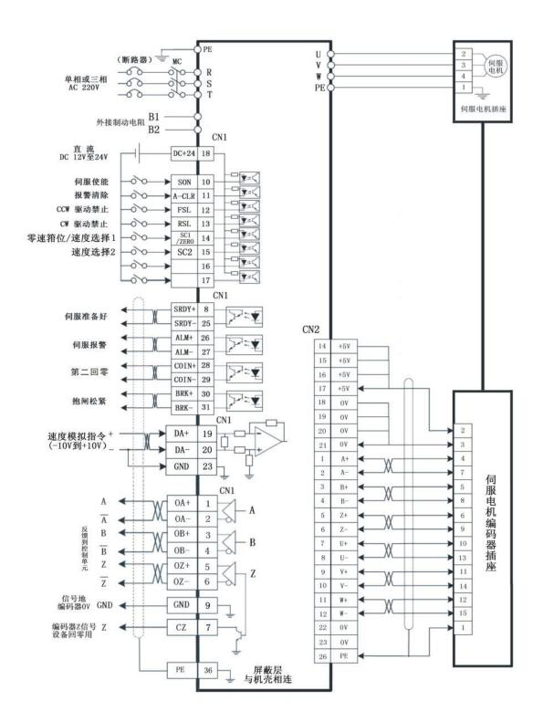
Figure 3.1 Wiring of Speed Control
