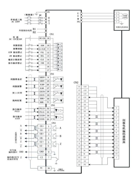
Figure 3.1 Wiring of Position Control
