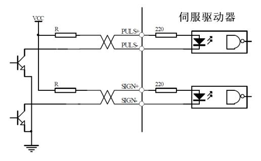
Figure 4.4-b Single-ended Output Mode of Pulse
