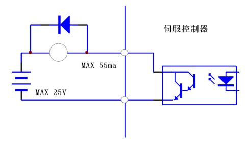
Figure 4.3-b Output Interface for Switching Value
