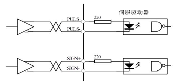
4.6 Principle of the Input Interface for Pulse Value
