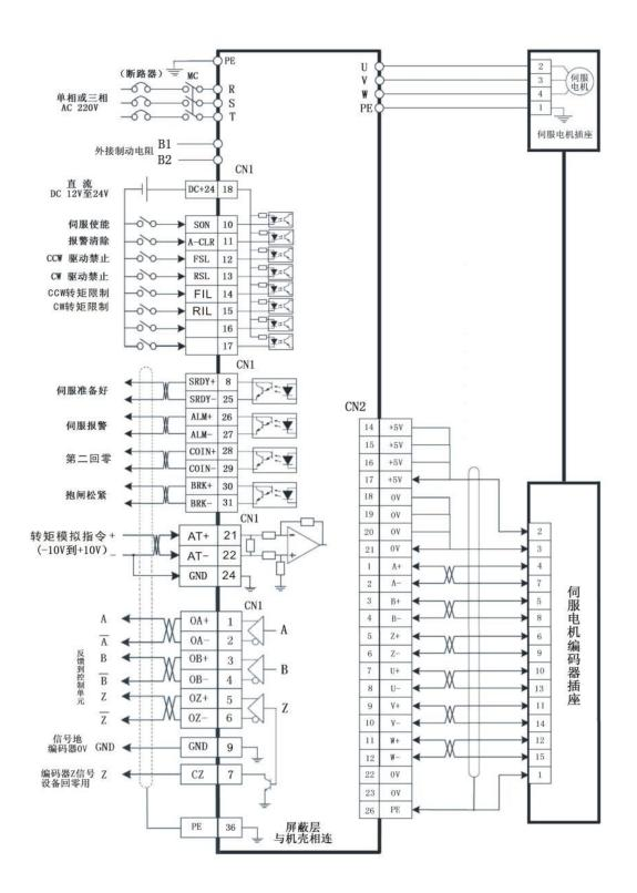
Figure 3.1 Wiring of Torque Control
