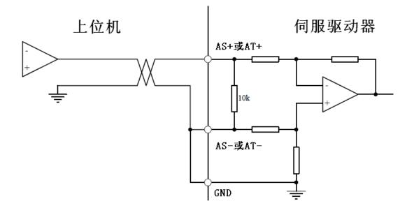
Figure 4.5-b Interface for Analog Single-ended Input
