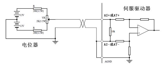
Figure 4.5-d Input Interface for Analog Single-ended Potentiometer
