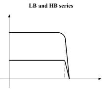
Mmax of LB and LBB series servo motor is equal to 3Mn; Mmax output status is the short time work of the servo motor. Please refer to the output capacity of the matching driver before use.
