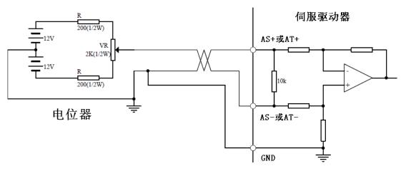
Figure 4.5-c Input Interface for Analog Differential Potentiometer
