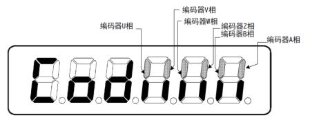
Figure 5.4 Status Display of Encoder Feedback Signal
