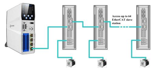
Figure 6.1 EM3E series network diagram
