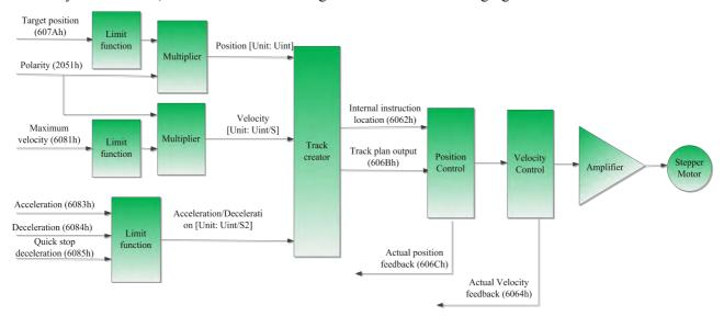
Figure 5.2 PP Mode control block diagram
