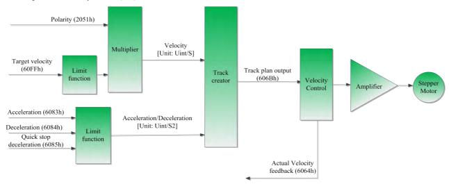
Figure 5.7 PV mode control block diagram
