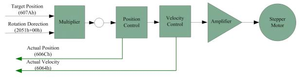
Figure 5.3 CSP Mode Diagram
