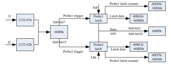
Figure 5.8 Touch probe function
