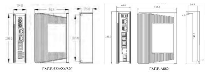
Figure 2.1 EM3E series mechanical drawing
