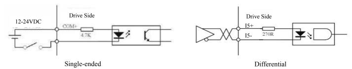
Figure 3.3 Input Interface Wiring
