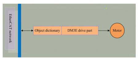
Figure 4.6: Object dictionary as access interface
