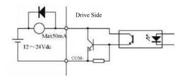
**Figure 3.4 Output Interface Wiring**
