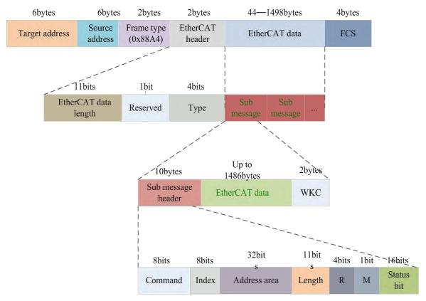
Figure 4.2: EtherCAT data frame structure
