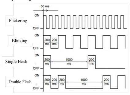
Figure 4.17: LED indicator lamp state
