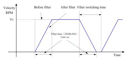
Figure 5.4 Filtering effect for square wave command
