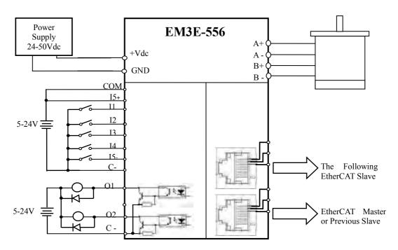
Figure 3.1 EM3E series wiring diagram
