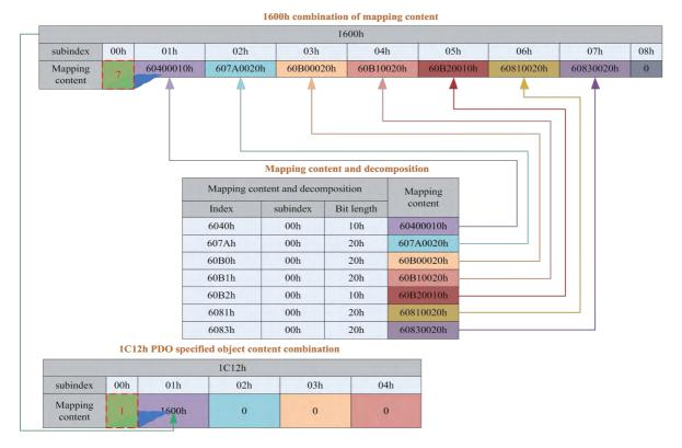
Figure 4.15: EM3E PDO dynamic mapping setting example overview
