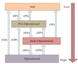
Figure 4.4: EtherCAT state machine transformation
