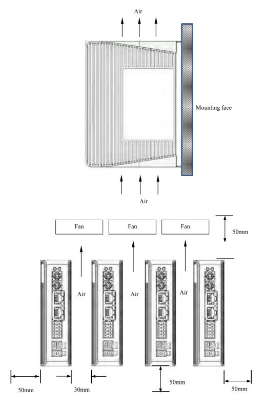
Figure 2.2 EM3E series installation drawing
