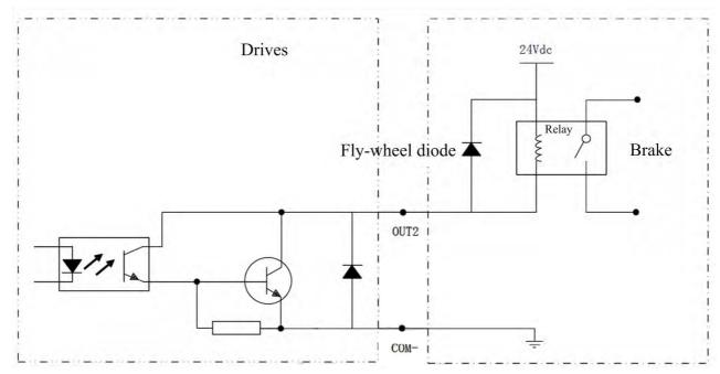
Figure 3.5 Brake Output Wiring
