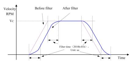
Figure 5.5 Filtering effect for trapezoidal wave command
