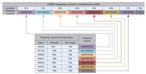
Figure 4.11: Set PDO mapping object content
