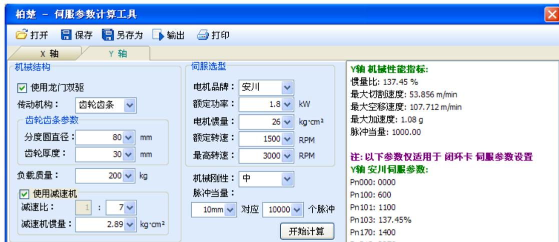
When inertia ratio is less than 200 percent, the device is light loaded, and enables high-speed cutting.
