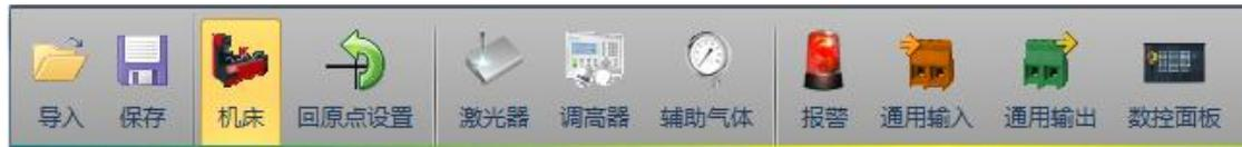
Top platform configuration tools are shortcut buttons to enter various parameter setting interface, such as machine and shortcut buttons of restoring origin setting as shown in Figure on the left; shortcut buttons of lasers during controlling the device, height controller and auxiliary gas as shown on the central; shortcut buttons of alarm, general input and output and numerical control panel as shown on the right.
