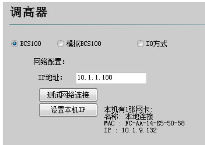
If use network height controller matched by our company (Abbreviation as BCS100), please set IP address which should be the same as the network address in the BCS 100 parameters.
