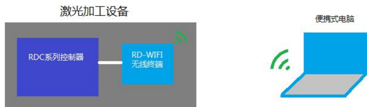
Figure-2 One laptop wireless connection diagram (Open WIFI)
