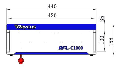
Figure 2 (a) Front view (Unit: mm)
