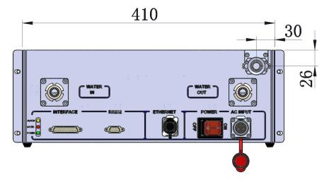
Figure 2 (b) Rear view (unit: mm)
