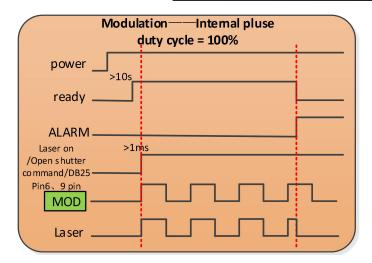
Figure 15 Modulation—sequence diagram
