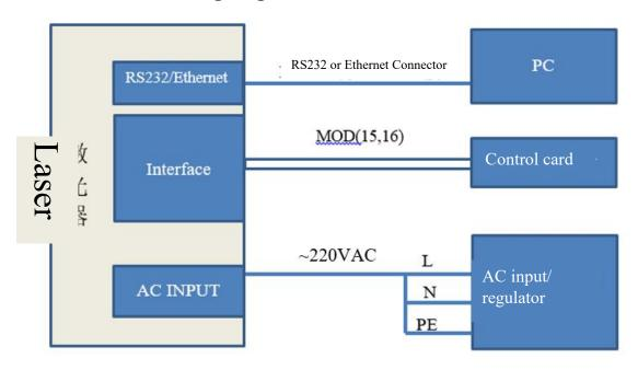
Figure 11 Wiring diagram in RS-232 mode
