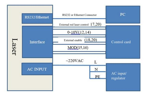
Figure 12 Wiring diagram in AD mode
