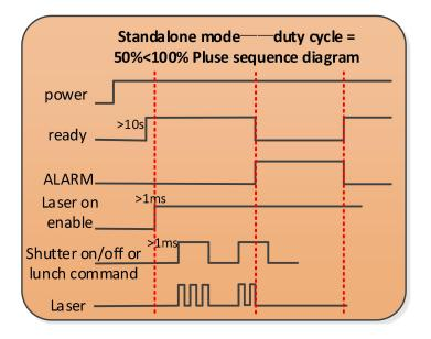
Figure 14 Standalone mode – Pluse sequence diagram
