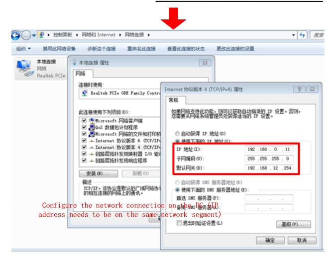
Figure 10 Ethernet connection steps
