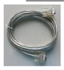
Figure 9 RS-232 serial cable
