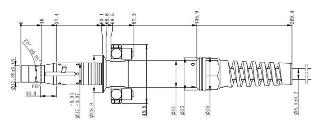
Figure 4 Dimensional drawing of welding IQB output optical cable
