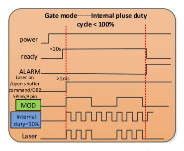
Figure 16 Gate mode – sequence diagram
