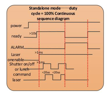
Figure 13 Standalone mode—Continuous sequence diagram
