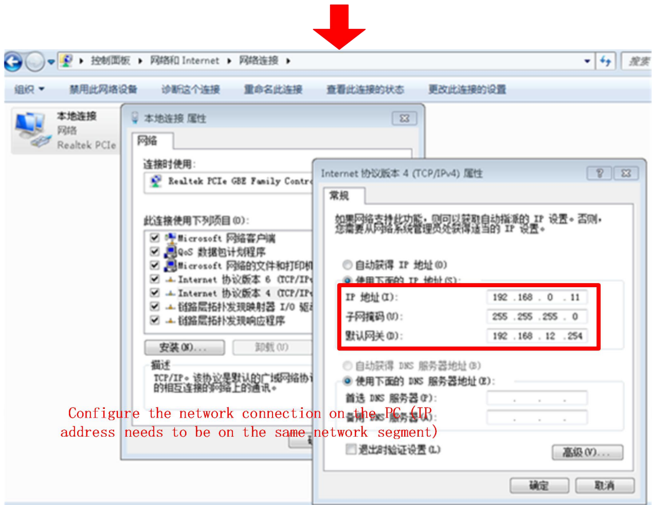
Figure 10 Ethernet connection steps
