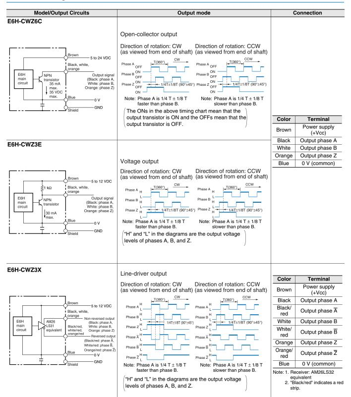
Note: Normally connect GND to 0 V or to an external ground.
