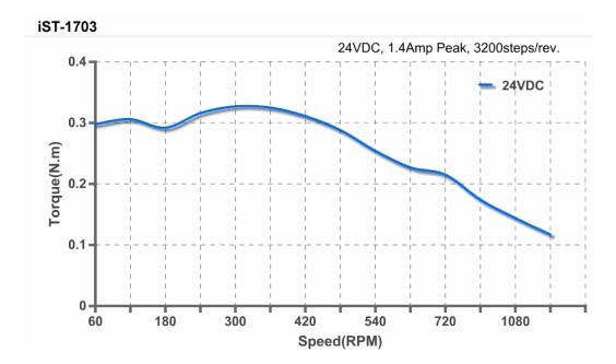
Note: The speed-torque curve is just for your reference.
