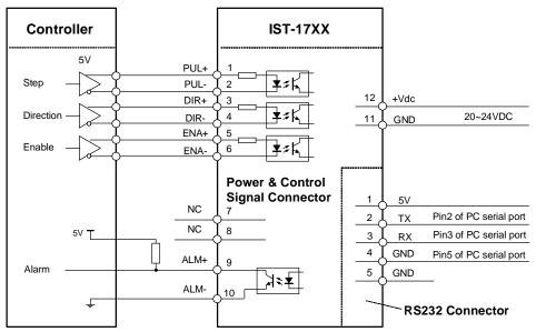
Connect IST-17XX to controller of differential output
