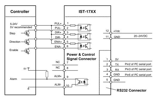
Connect IST-17XX to controller of sinking output
