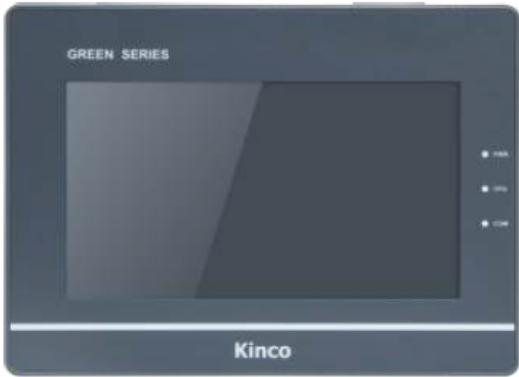
A dark blue Kinco HMI module with a rectangular screen. The screen displays a dark background with a diagonal line. Above the screen, the text "GREEN SERIES" is visible. Below the screen, the Kinco logo is present. On the right side of the module, there are three small indicator lights.  |
