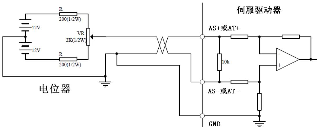
Figure 4.5-c Input Interface for Analog Differential Potentiometer
