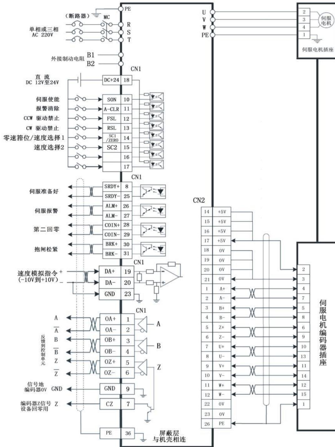
Figure 3.1 Wiring of Speed Control
