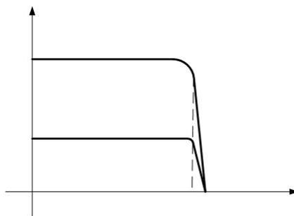
Mmax of LB and LBB series servo motor is equal to 3Mn; Mmax output status is the short time work of the servo motor. Please refer to the output capacity of the matching driver before use.
