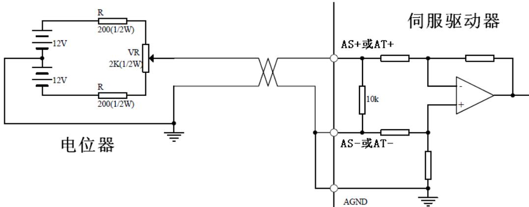
Figure 4.5-d Input Interface for Analog Single-ended Potentiometer
