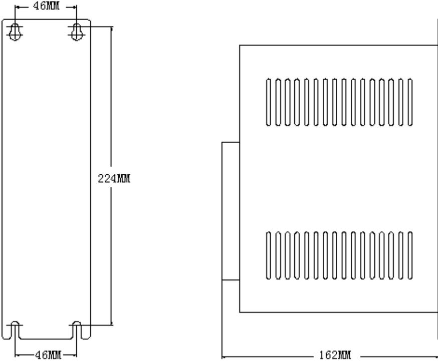
**Figure 1.21 Installation Dimensions
