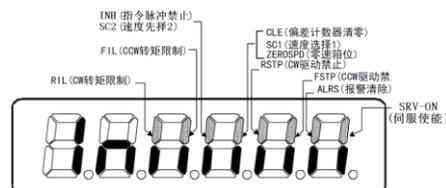
Figure 5.2 Display of Input Terminal Status
