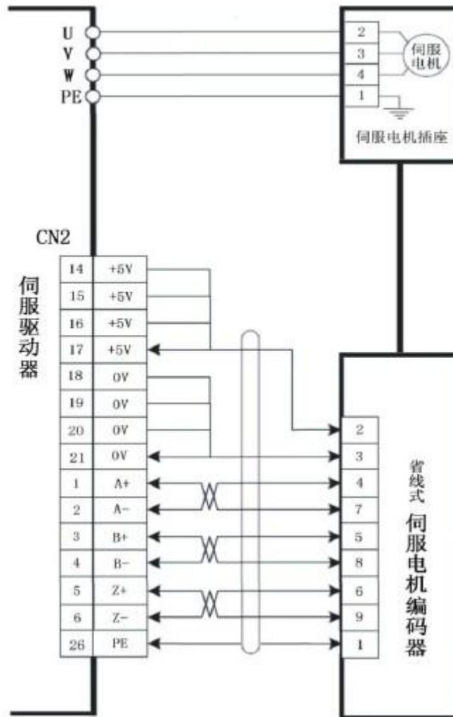
**Figure 3.4 Wiring Diagram for Wire Saving Motor Encoder**
