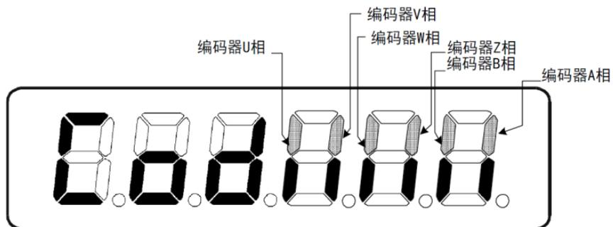
Figure 5.4 Status Display of Encoder Feedback Signal
