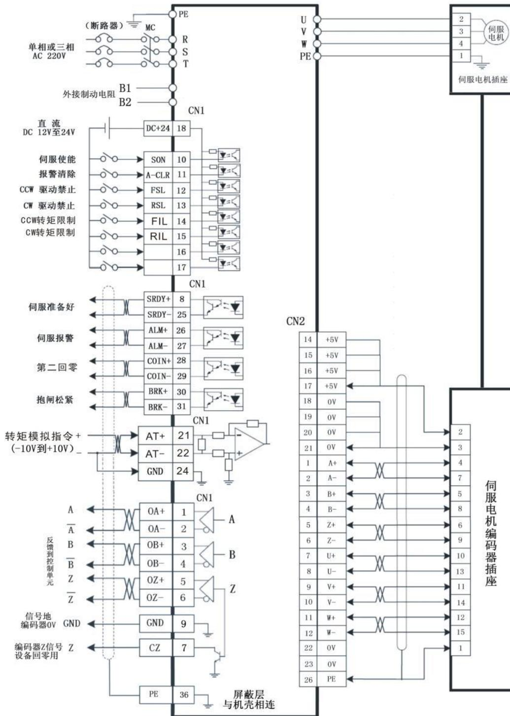
Figure 3.1 Wiring of Torque Control
