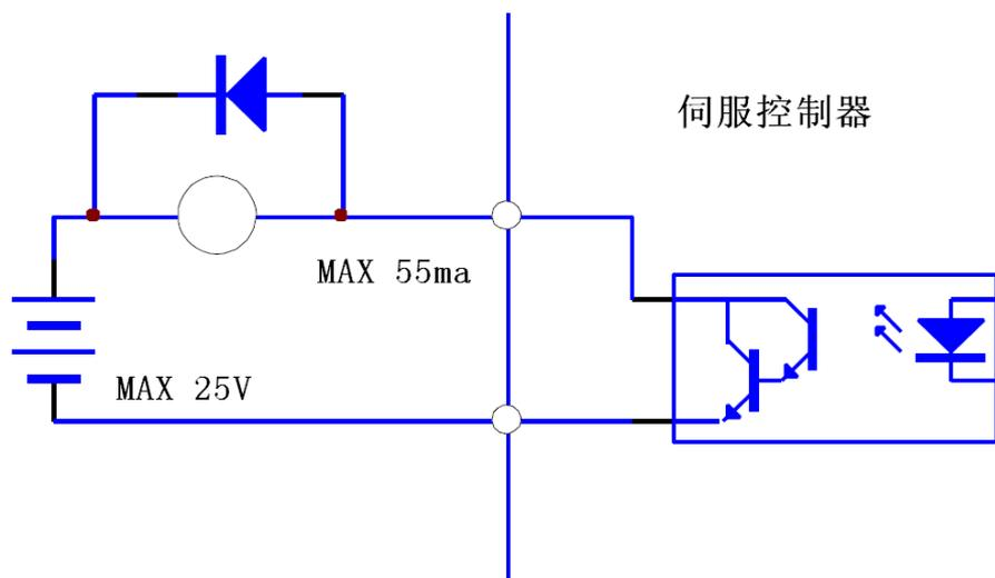
Figure 4.3-b Output Interface for Switching Value
