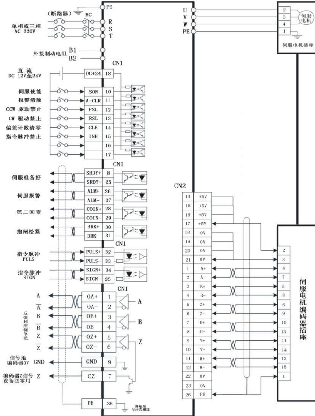
Figure 3.1 Wiring of Position Control
