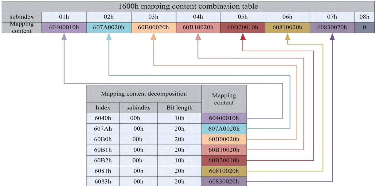
**Figure 4.11: Set PDO mapping object content**
