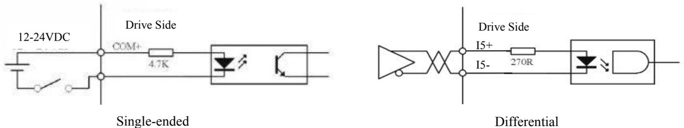
Figure 3.3 Input Interface Wiring
