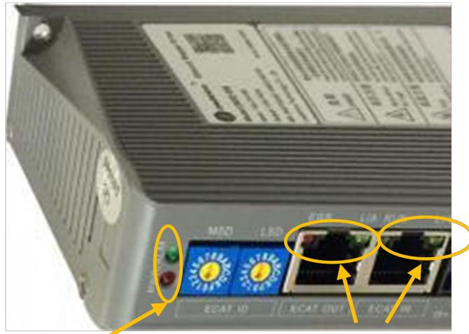
L1: Power/Alarm Indicator      L2: EtherCAT Communication Indicator
