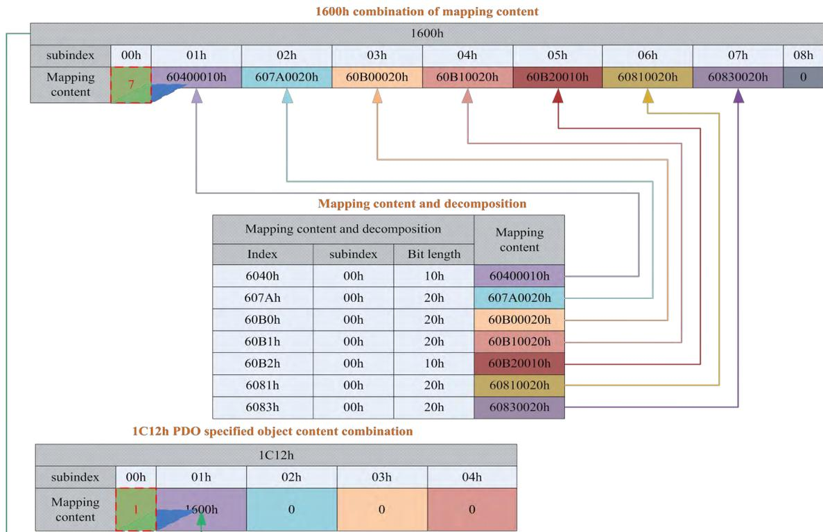
Figure 4.15: EM3E PDO dynamic mapping setting example overview
