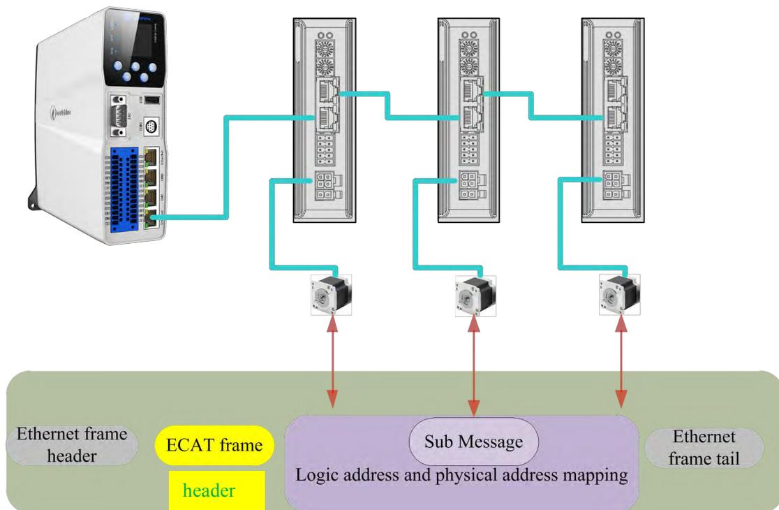
Figure 4.1: Digital packaging of process data
