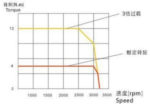
and high starting torque. Moreover, the maximum load that it withstands is three times higher than the rated torque of the related motor (when supplied by 3Ph-220Vac supply). it is pretty good on the occasions which the load has sudden fluctuations and is required to be re-started in work quickly.
