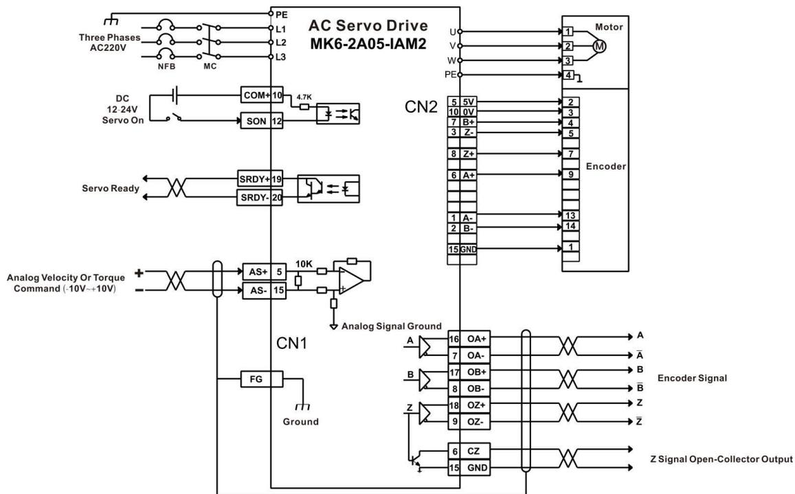
The wiring example (above) is for servo motors with flange size 60mm, 80mm and 90mm.
