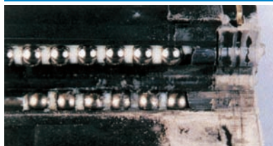
No. 1 Traveled 100 km (double-seal configuration)
