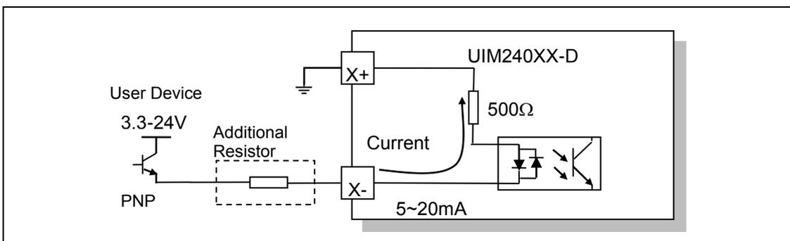
Note : X=4,5,6 in this figure, means terminal DIR , STP , ENA respectively.
