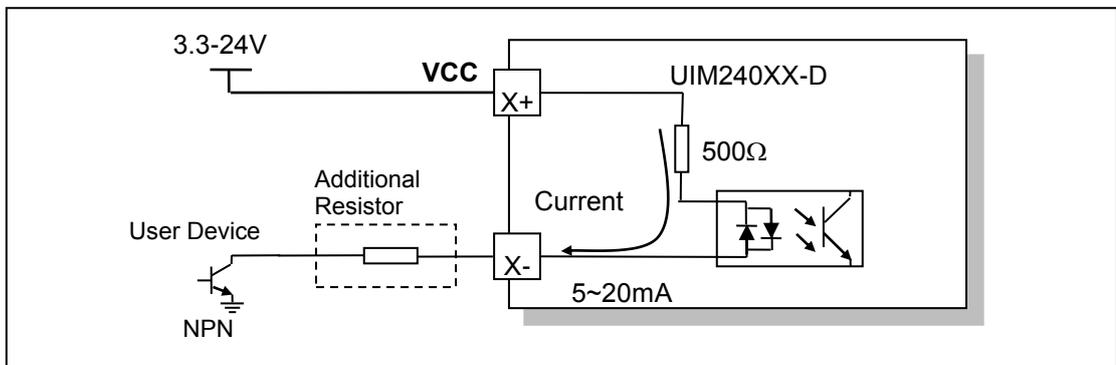
Note : X=4,5,6 in this figure, means terminal DIR , STP , ENA respectively.
