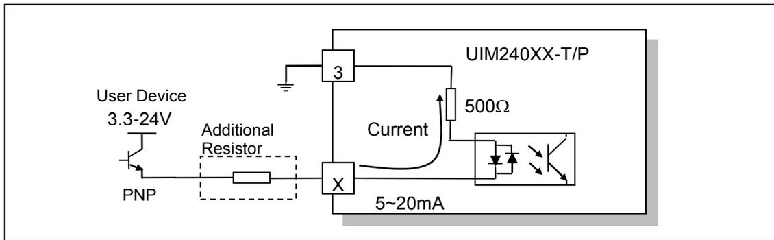
Note : X=4,5,6 in this figure, means terminal DIR , STP , ENA respectively.
