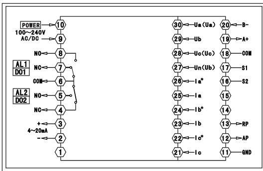
Note: ①Voltage input connection terminal,bracket terminals shows 3 phase 3 wire connection method, if there is any change, please turn to the correct diagram on the meter !
