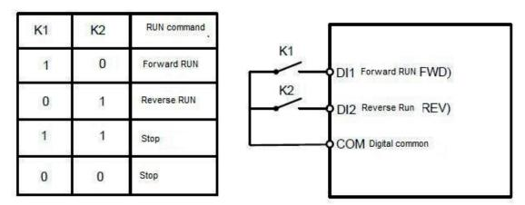
Figure 6-6 Setting of two-line mode 1
