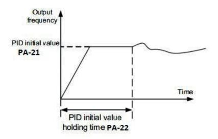
Figure 6-27 PID initial value function
