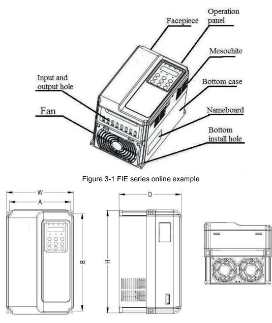
Figure 3-2 FIE series Plastic structure shape dimension and installation dimension sketch
