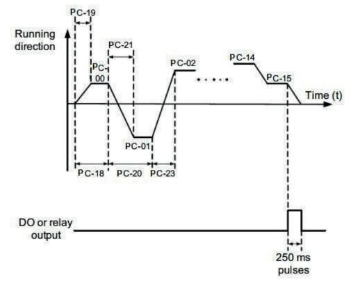
Figure 6-32 Simple PLC when used as frequency source
