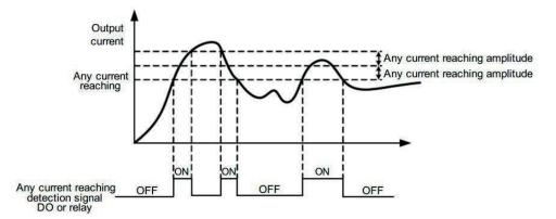
Figure 6-23 Any current reaching detection
