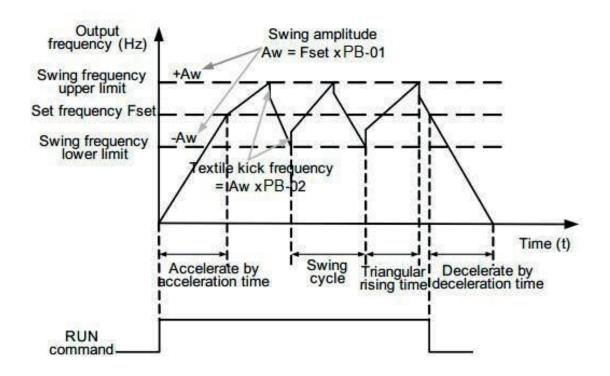
Figure 6-28 Swing frequency control
