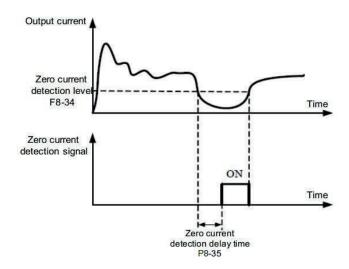
Figure 6-21 Zero current detection
