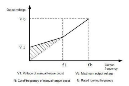
Figure 6-3 Manual torque boost
