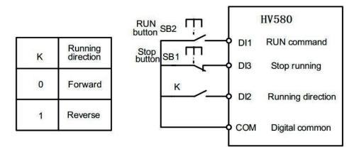
Figure 6-9 Setting of three-line mode 2
