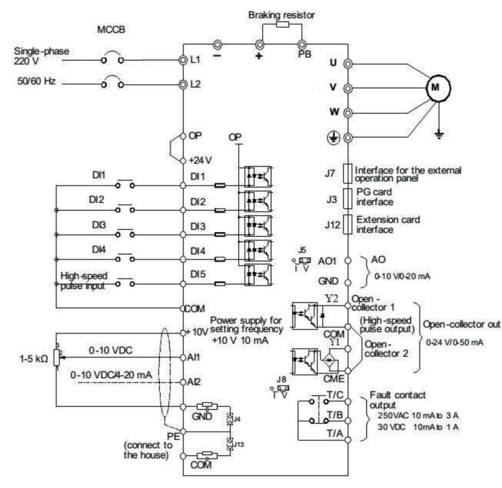
Figure 3-7 AC drives control circuit connection mode
