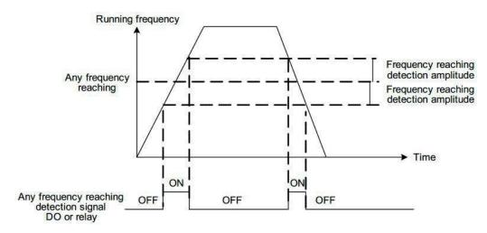
Figure 6-20 Any frequency reaching detection
