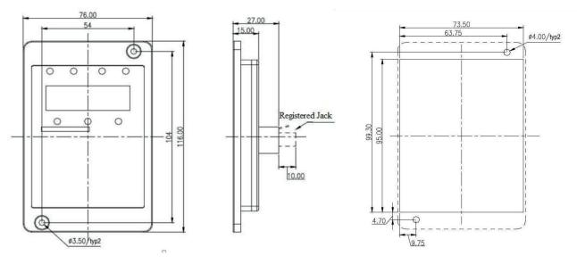
Figure 3-3 keyboard installation dimensions
