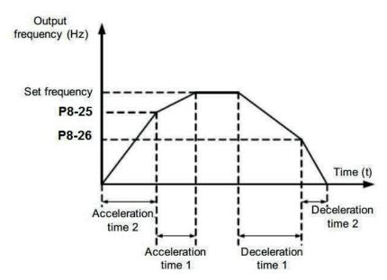
Figure 6-19 Acceleration/deceleration time switchovers
