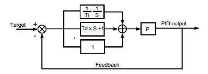
Figure 6-25 Principle block diagram of PID control
