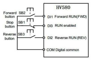
Figure 6-8 Setting of three-line mode 1
