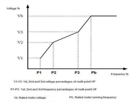
Figure 6-4 Setting of multi-point VF curve
