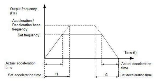
Figure 6-1 Acceleration / Deceleration time
