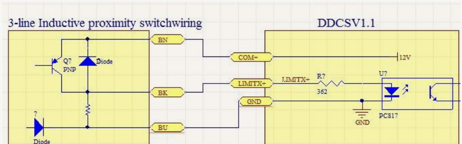
Pic.2-20 3-line Inductive proximity switchwiring mode
